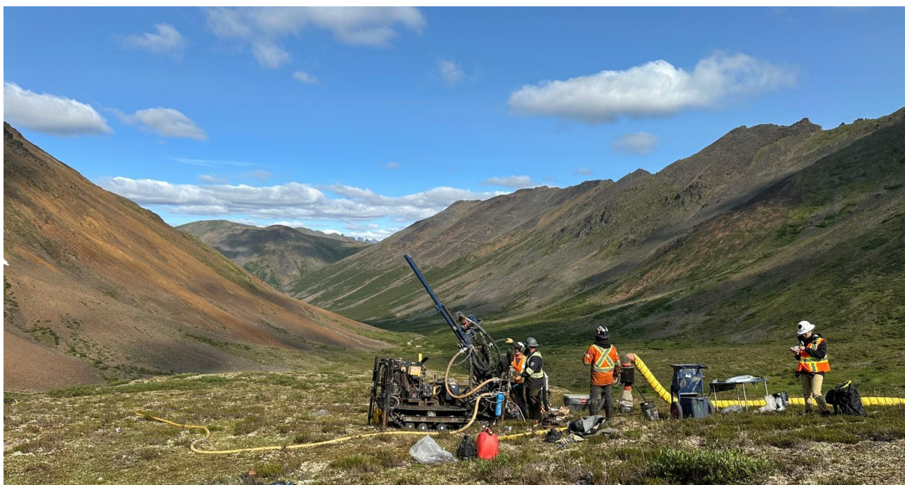
Figure 5: RAB rig set up at the Rainbow Prospect, Aurora Project. Note extensive iron oxide staining.
