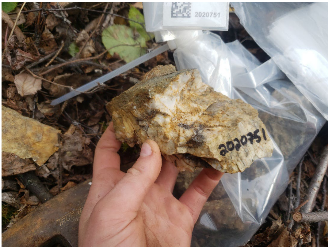
Figure 4A: Rock samples from historical trenches along strike from the Shanghai Silver Mine (Keno Hill-style mineralization). Sample 2020751 shows schist - shale type host with quartz veins, sulphosalts, stockwork veining, oxidized sulphide, and grey sulphide.
