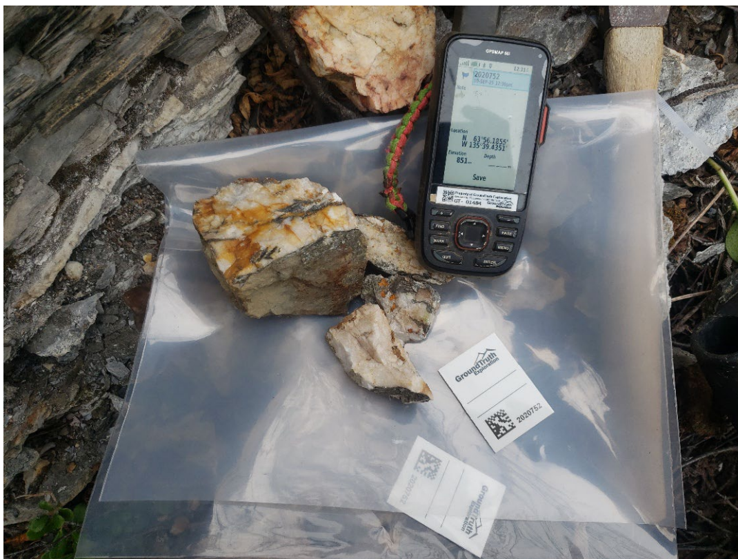
Figure 4B: Rock samples from historical trenches along strike from the Shanghai Silver Mine (Keno Hill-style mineralization). Sample 2020752 shows milky white quartz veins within dark grey schist/shale host. Veins have rusty spots and vugs of ex-sulphide.
